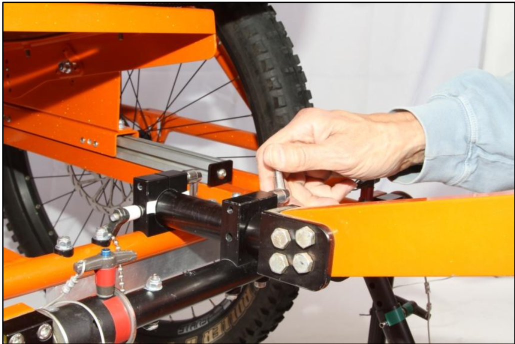
Figure 40. Clamping the forward beam in place.
