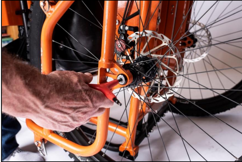
Figure 23. Tighten the axle with a 6mm hex wrench.
