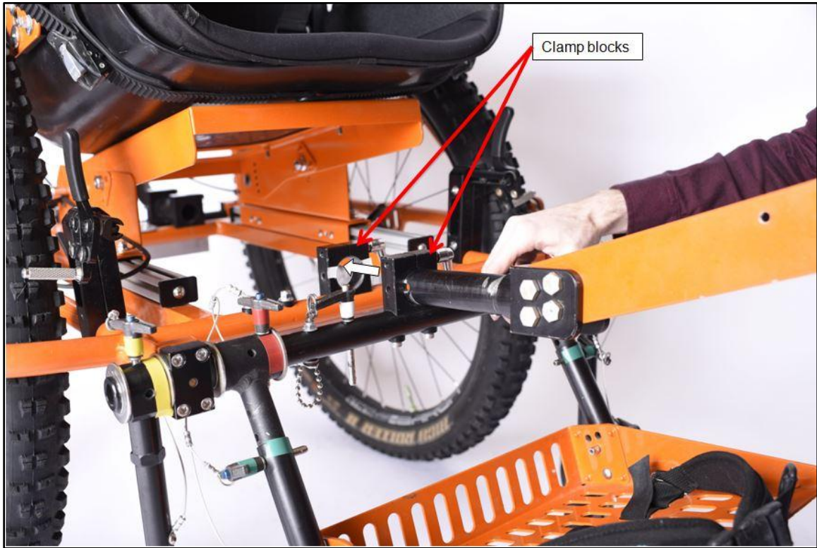
Figure 38. Sliding the rear, round end of the forward beam into the clamp blocks.
