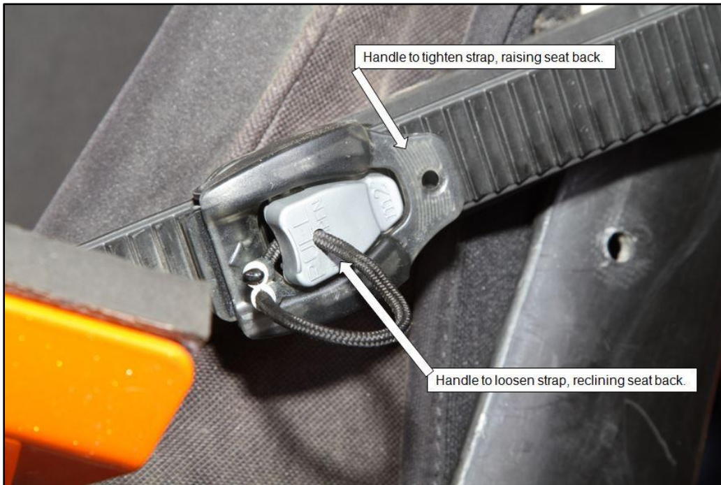
Figure 45. Buckle for adjusting the angle of the seatback.
