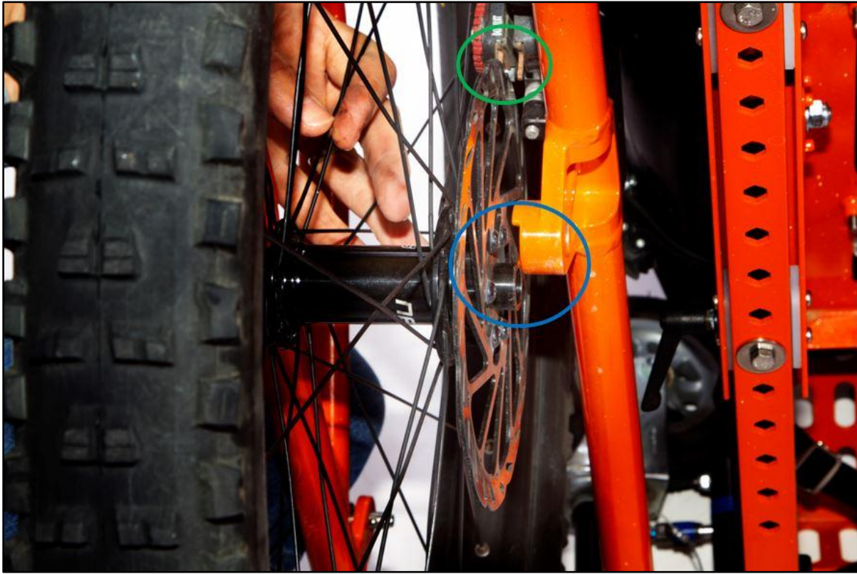
Figure 21. Wheel placed in the axle dropouts with the brake rotor in the brake rotor slot.
