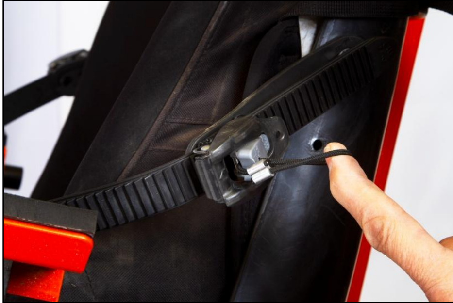
Figure 46. Adjusting the seatback position: Recline the seatback.
