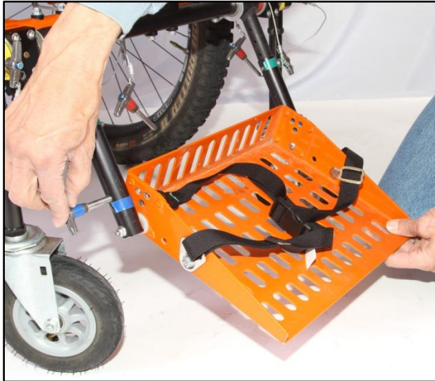
Figure 30. Unpin the blue pins from both sides of the footrest tray.
