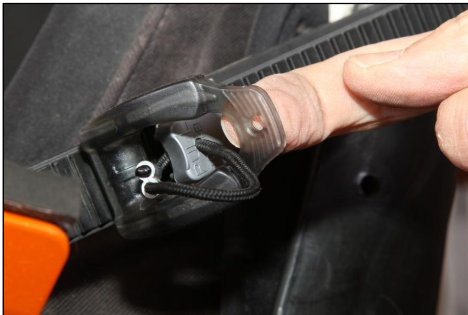
Figure 47. Adjusting the seatback position: Raising the seatback.
