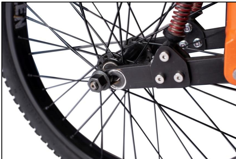
Figure 35. Installing the front wheel on the forward beam.
