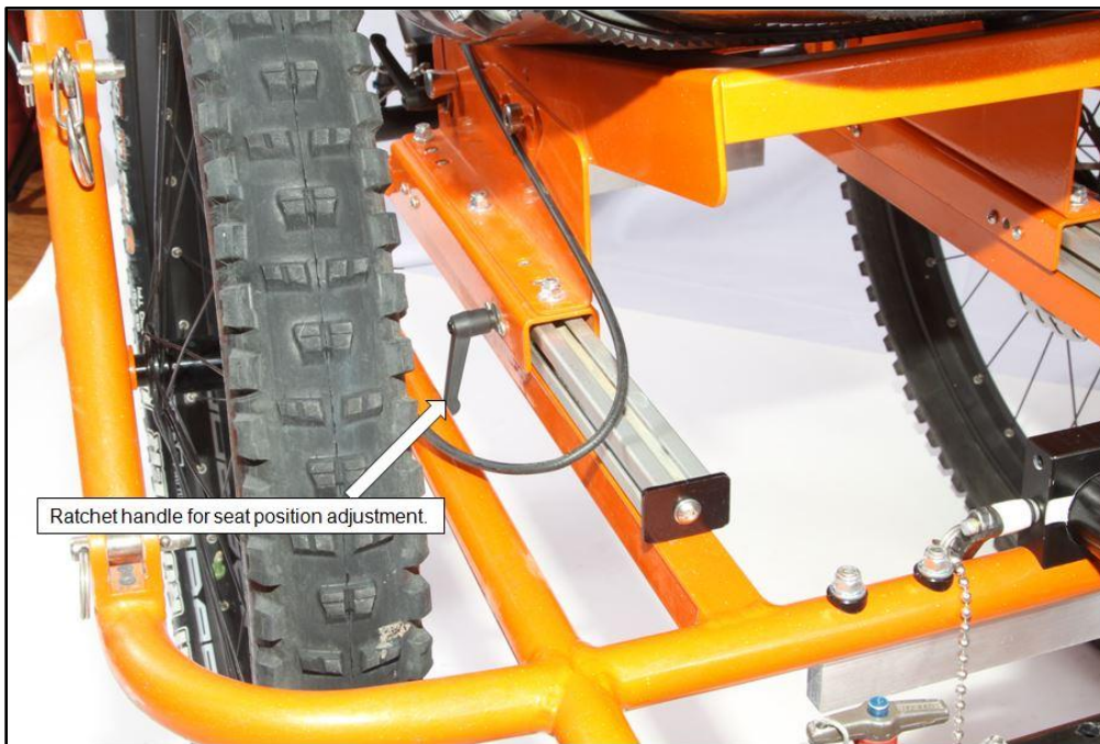
Figure 43. Ratchet handle for adjusting seat position.
