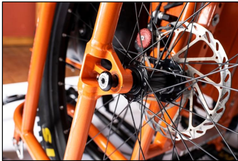
Figure 22. Axle placed through hub and ready to be tightened.
