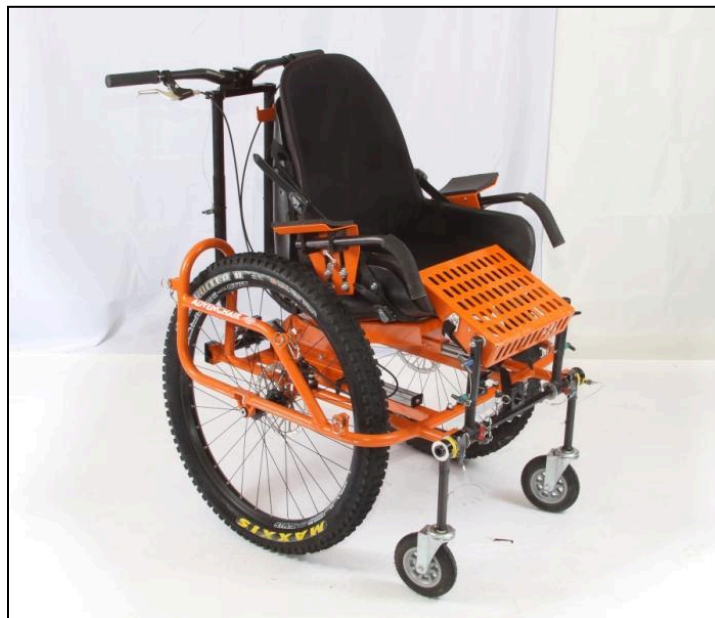
Figure 26. AdvenChair with main wheels and casters in place and seatback raised.
