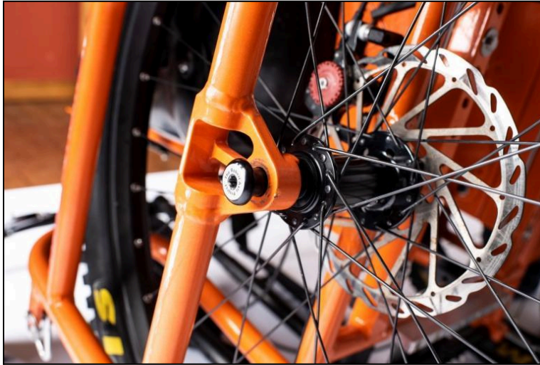
Figure 22. Axle placed through the hub and ready to be tightened.
