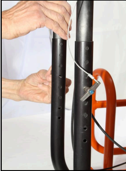
Figure 18. Pin handlebars in place.
