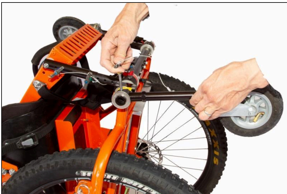
Figure 25. Lower the casters into wheelchair mode.
