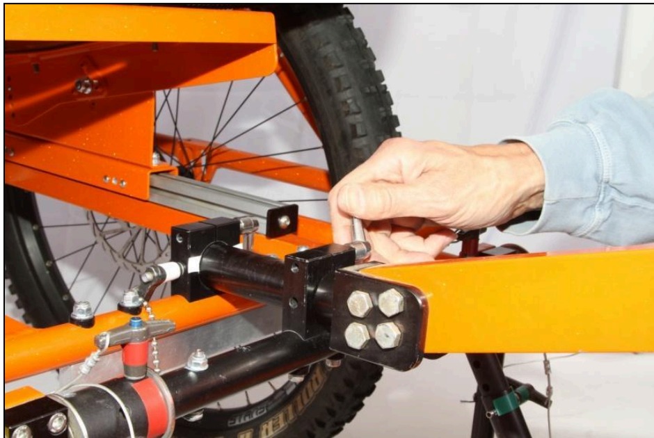
Figure 40. Clamping the forward beam in place.
