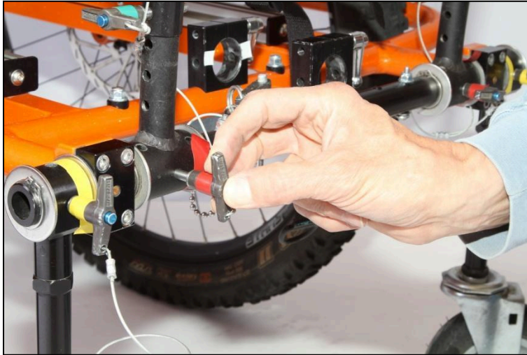
Figure 29. Use the red detent pins to position the footrest assembly.
