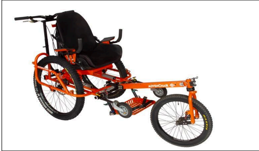
Figure 41. Casters up and the AdvenChair in all-terrain mode.
