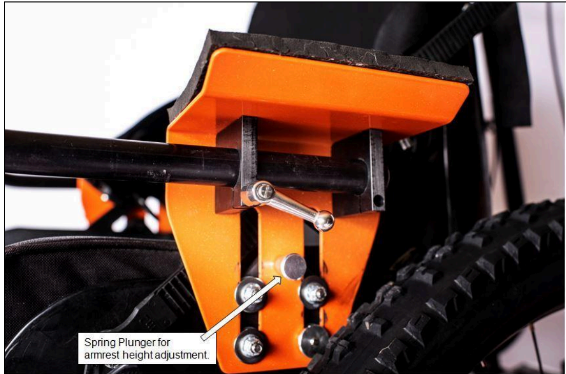
Figure 48. Spring plunger used to adjust the height of the armrests.
